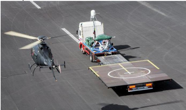
Figure 29. Landing on a moving platform. Measured signals were correlated with particular approaches to make them easier to interpret. Example of flight test data with distinguished approaches is shown on Figure 30. Following graphs represents signals 800.0, 801.0 911.3, 800.8, 811.8 (refer to Table 4). Additionally, video recording of each particular approach was provided.
