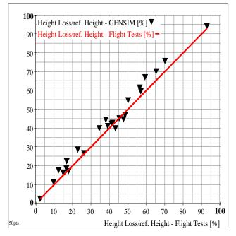
Figure 18: OEI flyaway height loss. Comparison between GENSIM and flight tests results.
