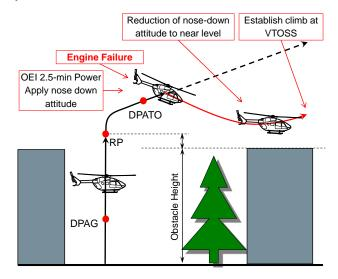
Figure 6: PC2 DLE: OEI after RP, continued takeoff procedure.
