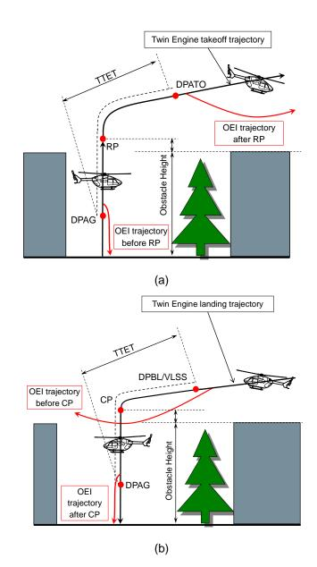
Figure 3: Helipad PC2 DLE definitions: takeoff (a) and landing (b).
