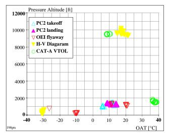
Figure 11: flight tests envelope considered for the establishment of PC2 DLE performance.
