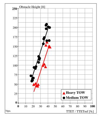
Figure 12: PC2 DLE exposure time approximation based on flight data. TETT represented in normalized form.
