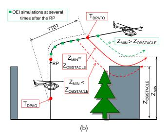
Figure 19: Exposure time determination. Before RP (a) and after RP (b).
