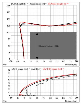
Figure 15: PC2 AEO takeoff with vertical procedure. Comparison GENSIM against flight test data.
