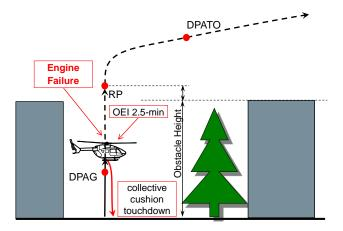
Figure 5: PC2 DLE: OEI prior to RP, aborted takeoff procedure.
