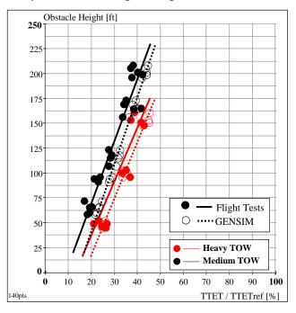
Figure 16: PC2 DLE normalized exposure time approximation based on flight data and comparison against GENSIM simulation results.
