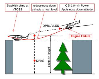
Figure 8: PC2 DLE: OEI prior to CP, balked landing procedure.
