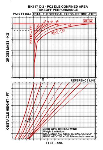
Figure 20: Example of FLM chart for confined helipad PC2 DLE takeoff in sea level (SL).
