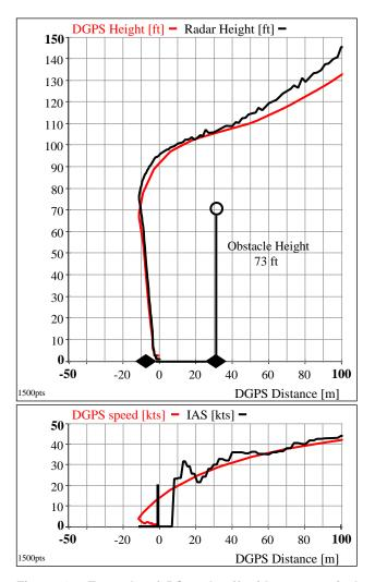
Figure 10: Example of PC2 takeoff with near vertical procedure.
