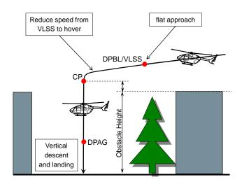
Figure 7: PC2 DLE: normal AEO landing procedure.
