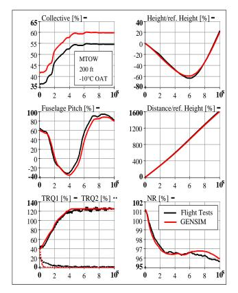
Figure 17: Time History of an OEI flyaway. Comparison between GENSIM and flight test data.
