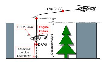
Figure 9: PC2 DLE: OEI after CP, continued landing procedure.
