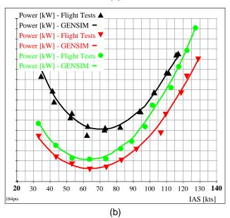
Figure 14: BK117 C-2 steady state performance; comparison between flight test data and GENSIM simulations for (a) HOGE and (b) forward flight.
