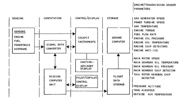
Fig. 14: Monitoring flow diagram
