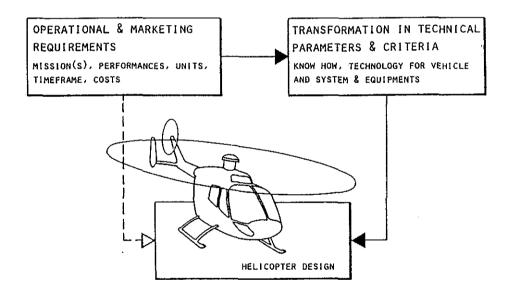
Fig. 1: Impacts on overall helicopter design
