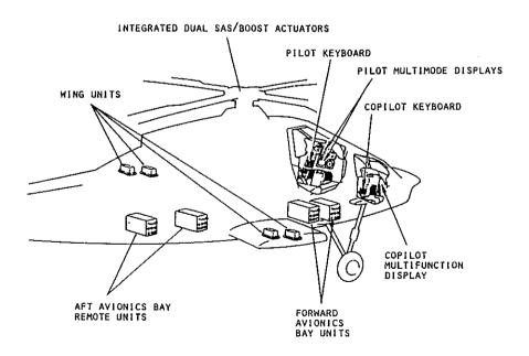
Fig. 23: Remoted terminal units installation
