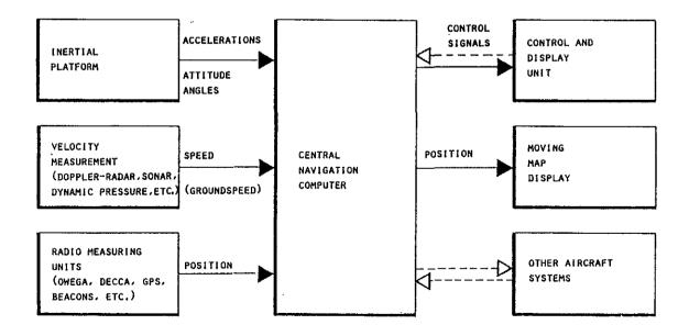
Fig. 7: Integrated navigation system diagram
