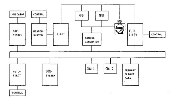
Fig. 17: Multiplex bus system architecture
