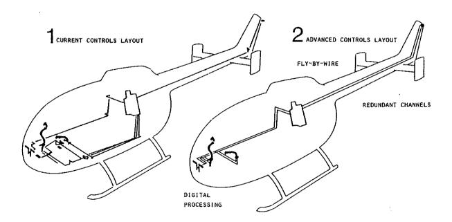
Fig. 15: Comparison mechanical - electronic flight controls
