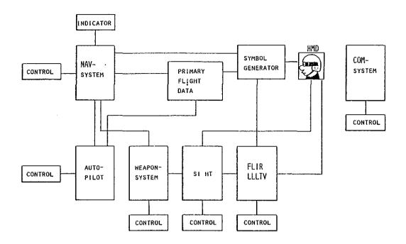
Fig. 16: Conventional system architecture
