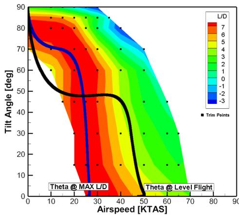
Figure 20: Transition simulation and GAVM L/D contours
