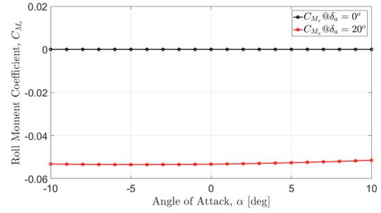
Figure 11: Roll moment coefficient variation with angle of attack
