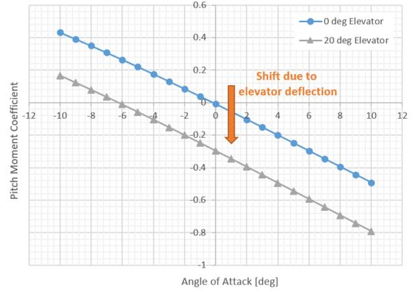
Figure 7: Shift in pitch moment due to a deflected elevator
