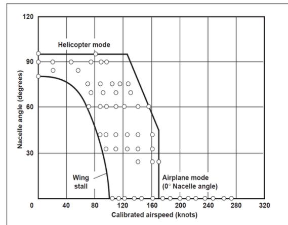
Figure 1: Conversion corridor of the XV-15 tilt rotor research aircraft<sup>1</sup>
