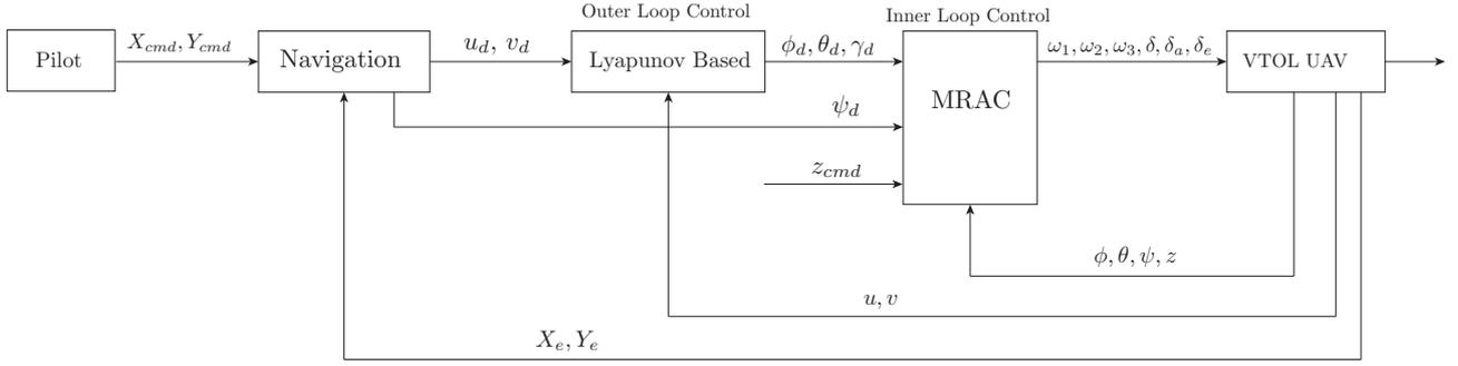
Figure 12: Block Diagram for Position Control Architecture
