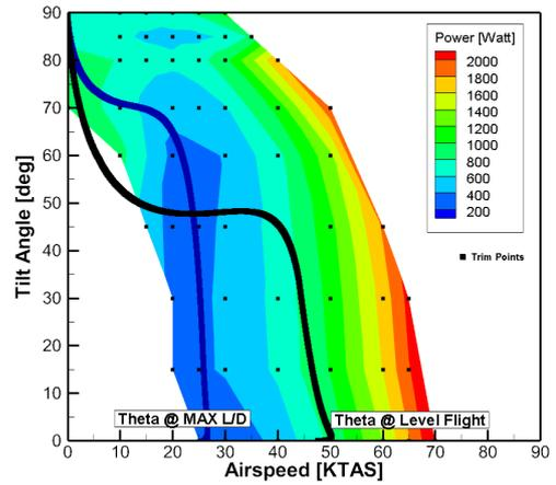
Figure 21: Transition simulation and GAVM required power contours
