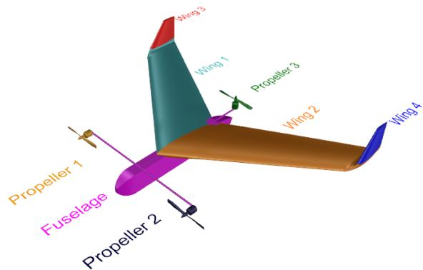
Figure 4: GAVM Components Utilized in Nonlinear Model
