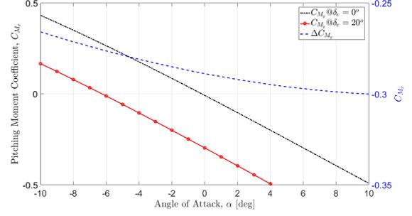
Figure 10: Pitching moment coefficient variation with angle of attack
