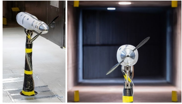
Figure 10. Isolated propeller model in the wind tunnel
