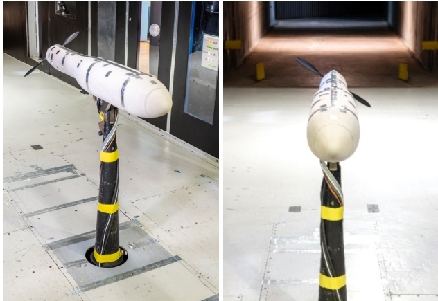
Figure 9. Pusher propeller model in the wind tunnel
