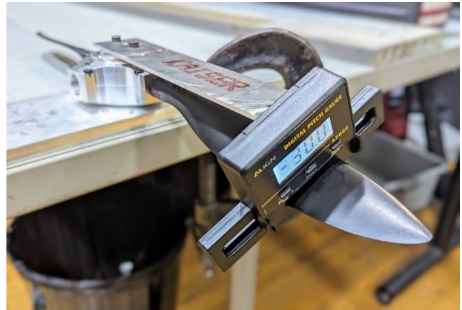
Figure 8. Setting the collective pitch angle at 75% radius (tractor orientation)
