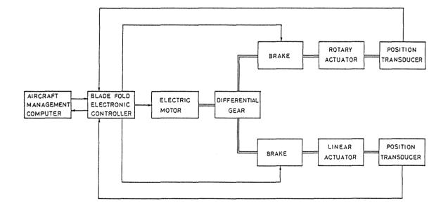
FIG. 5 SCHEMATIC OF AN ELECTRONICALLY CONTROLLED BLADE FOLD ACTUATOR
