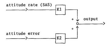
If the attitude error increases, the possibility exists that after multiplication by K2, the attitude error contribution could saturate. The SAS will no longer have complete control of the output, the result being a partially undamped system. In this situation, the A129 verified a divergent control. A possible solution might be:
