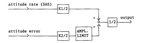
By selecting the amplitude limit threshold to equal half of allowed digital range, the attitude error path will not lose any dynamic quality (with respect to the previous implementation), and thereby the SAS can have complete control of the output signal.
