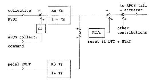
The collective stick position (provided by RVDT sensors), plus the AFCS collective command, together determine the total amount of main rotor collective. The first block encountered, after the two signal addition, provides an output proportional to the collective variation which decays to zero with a time constant equal to  $\tau$ . During this time, the integrator K2/s charges. By selecting the proper gains, the response will be proportional to the collective input:
