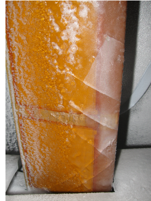
Figure 5: Rotor blade with accreted ice and spontaneous cracks in the ice due to torsion deformation
