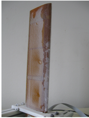
Figure 3: Blade segment with accreted ice at the leading edge
