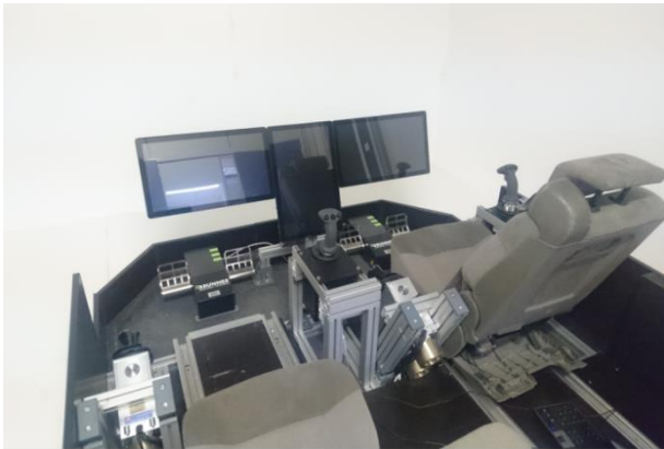
Figure 2: PycsHel simulator in dual pilot configuration, integrating Safran E&D ASSU (collectives)
