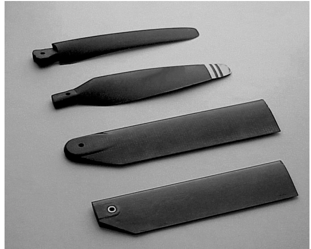
Fig. 3. From top to bottom, 3-bladed model, twisted-small-chord, twisted-large-chord, untwisted blades and 2-bladed model untwisted blade from Ref. 7.
