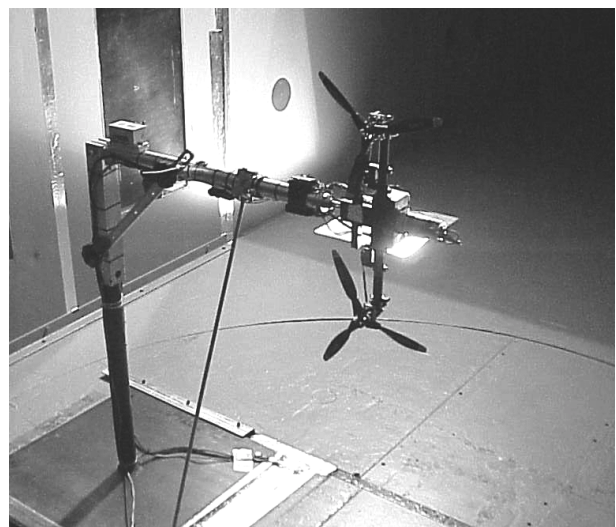
Fig. 1. Tiltrotor Descent Aerodynamics test in the Ames 7- by 10- Foot Wind Tunnel.
