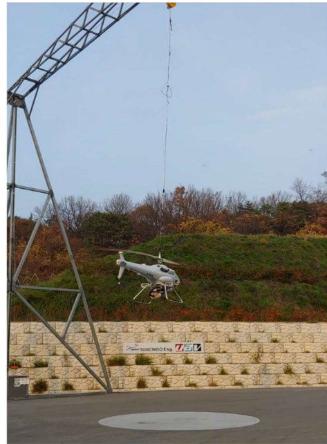
Figure 7: Safety wire test before MPUH flight test
