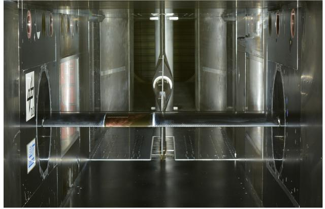
Figure 1: DSA-9A airfoil model in the Transonic Wind Tunnel Goettingen.
