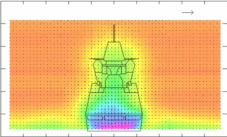
Figure 3: Wind tunnel wake rake measurements (local airspeed disturbance)
