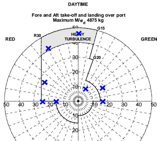
Figure 10: Test points piloted simulation session [1]
