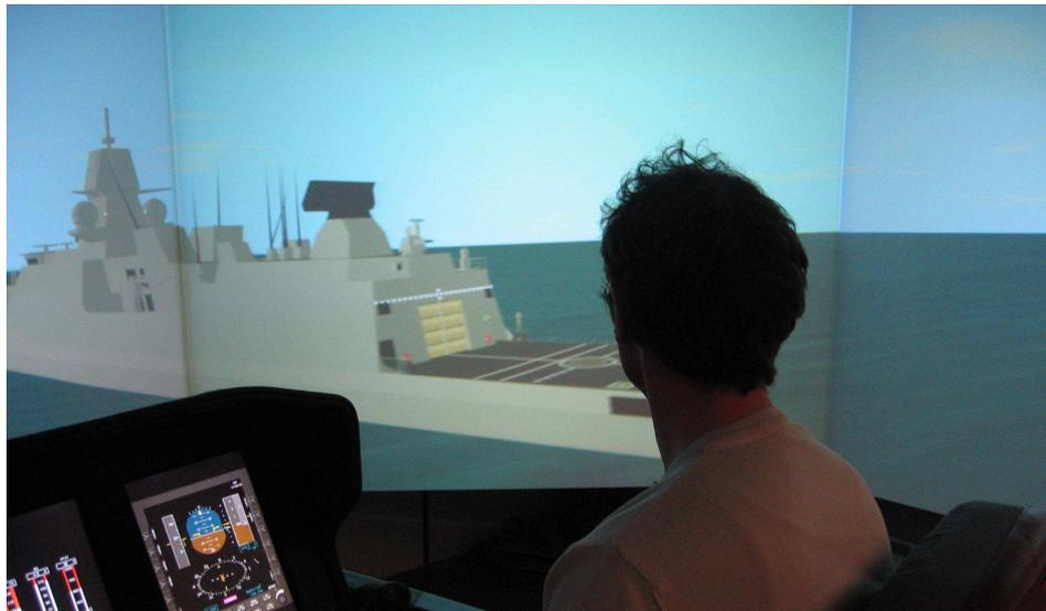
*Figure 8: RNLN test pilot performing a fore-aft approach over port*
