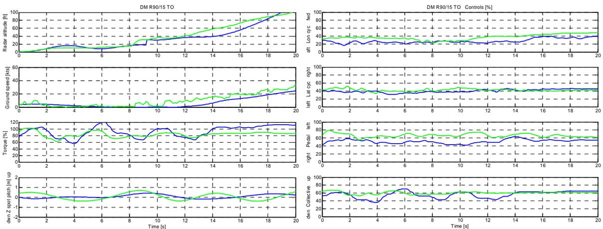
Figure 12: Take-off over port, HPS session (blue) and flight test (green) for R90/15.
