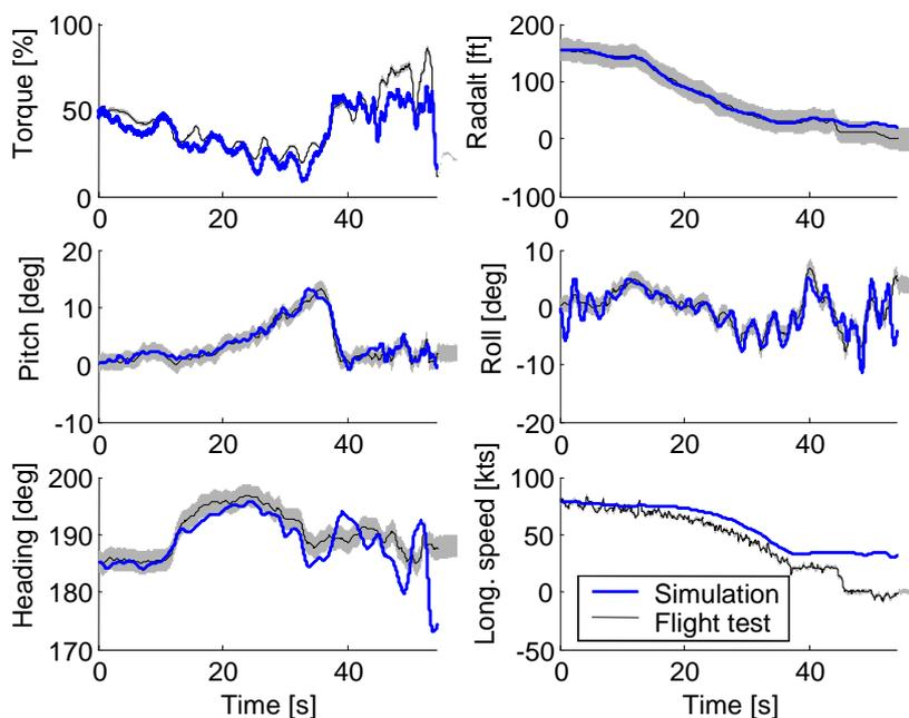
Figure 7: Match of off-line simulation with flight test for a FAP approach.
