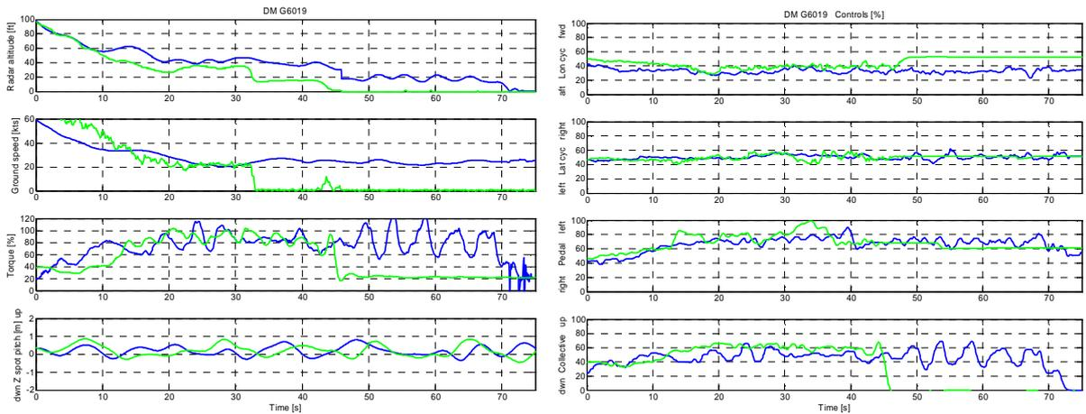
Figure 11: Landing over port, HPS session (blue) and flight test (green) for G60/19.
