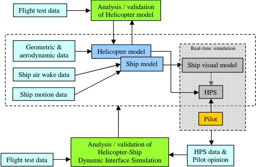
Figure 2: Development of the helicopter-ship dynamic interface simulation
