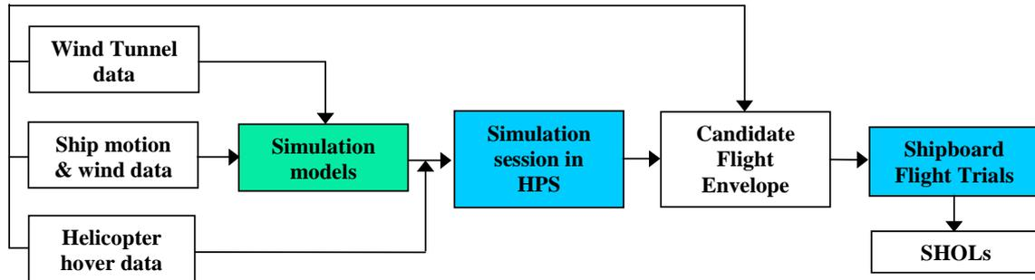
Figure 13: Contribution of simulation to SHOL determination.
