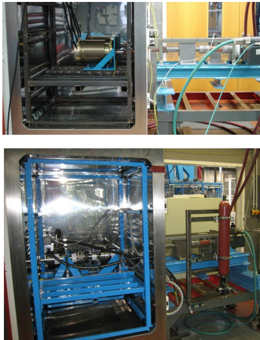
Figure 5: Validation of Thermal Behavior and Low Temperature Performance of Electrical Machine (Top) and Actuator Gearbox (Bottom)
