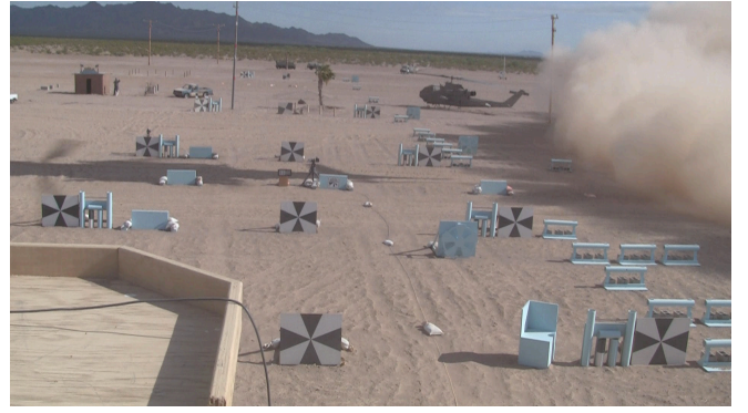
Fig. 5: Locations utilized for MTF extraction over a broad field of view.
