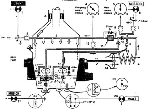
Figure 8 Main Gear Box Lubrication System
