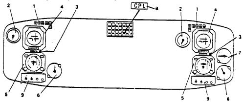
Figure 3 Autopilot and Related Systems on the Instrument Panel
