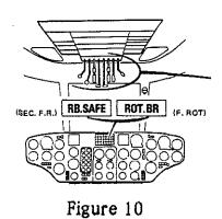
The Super Puma has a two-lever rotor brake system, the rotor brake safe lever and the rotor brake lever. It is possible to move the rotor brake to the braking position in flight (which obviously should <u>not</u> be done), but it will do nothing more than cause the "ROT.BR" light to illuminate. You can only obtain rotor braking when both levers are pushed forward, a sensible system which just about guarantees that the rotor brake won't be engaged inadvertently at the wrong time.
