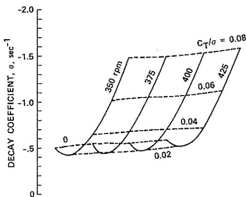
Figure 15. Predicted damping as a function of rotor rotation rate and thrust: dynamic inflow model.
