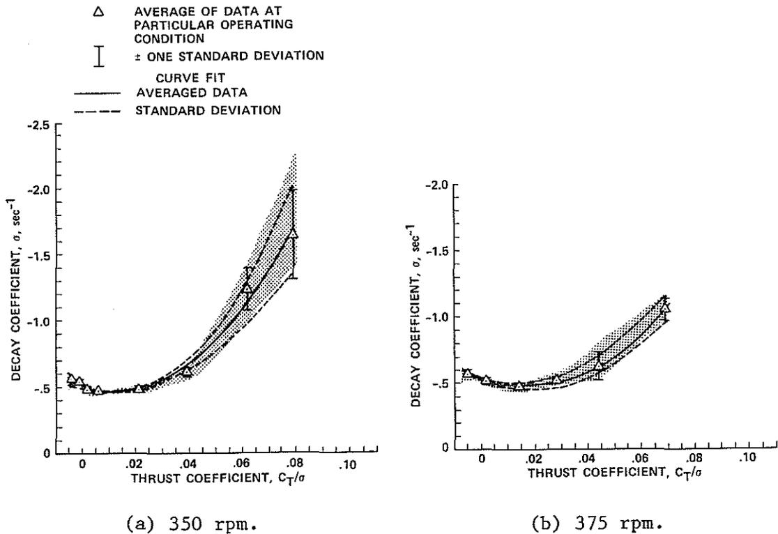
Figure 11. Polynomial curve fit of average regressing inplane modal damping data at each operating condition.
