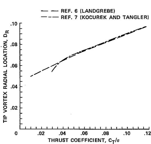
(a) Radial location inboard from blade tip ( $\div R$ ).
