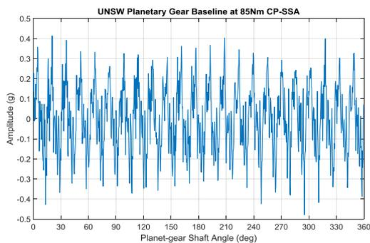
Figure 5. Baseline CP-SSA at 85 NM torque for the test gearbox
