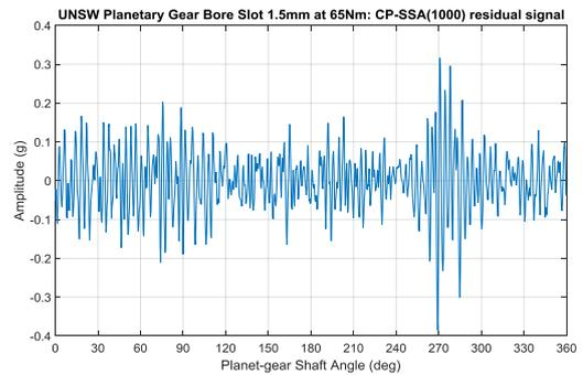
**Figure 12.** Planet gear residual signal for 1.5mm notch at 65Nm torque where  $RMS = 0.0767(g)$ ,  $Kurt = 4.788$
