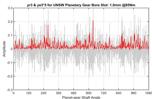
Figure 19. Residual (grey) and scaled envelope (red) signals for 1.0 mm notch at 85 Nm torque
