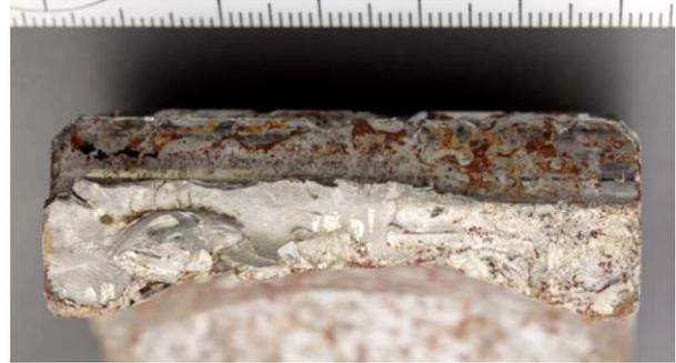
*Figure 1. H225 Super Puma planet gear bore crack propagation [2, Fig. 31] – Photo from AIBN/QinetiQ*
