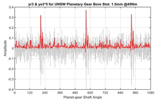
Figure 20. Residual (grey) and scaled envelope (red) signals for 1.5 mm notch at 45 Nm torque
