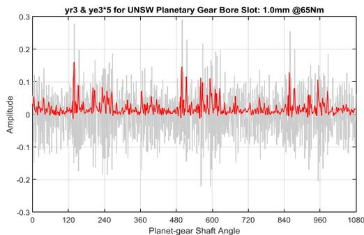
Figure 18. Residual (grey) and scaled envelope (red) signals for 1.0 mm notch at 65 Nm torque
