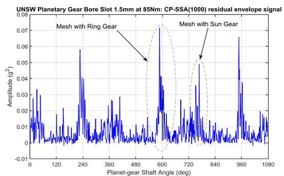
Figure 16. Feature signal (in 3 revolutions) for the detection of planet gear bore cracking. It is assumed that the larger spike is the mesh with the ring gear, and the smaller one is with the sun gear
