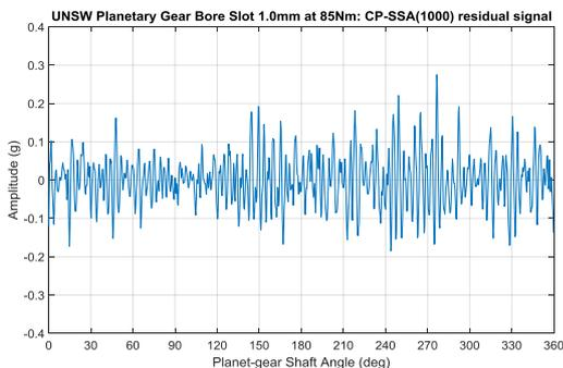
**Figure 10.** Planet gear residual signal for 1.0mm notch at 85Nm torque where  $RMS = 0.067(g)$ ,  $Kurt = 3.66$
