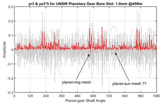
Figure 17. Residual (grey) and scaled envelope (red) signals for 1.0 mm notch at 45 Nm torque
