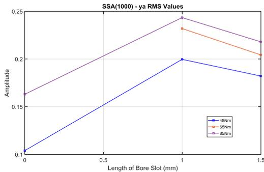
Figure 14. Trending of RMS values of CP-SSA signals
