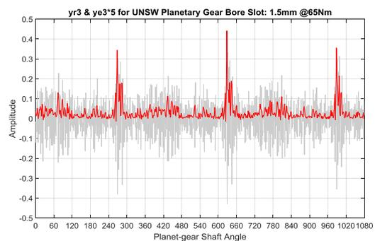
Figure 21. Residual (grey) and scaled envelope (red) signals for 1.5 mm notch at 65 Nm torque
