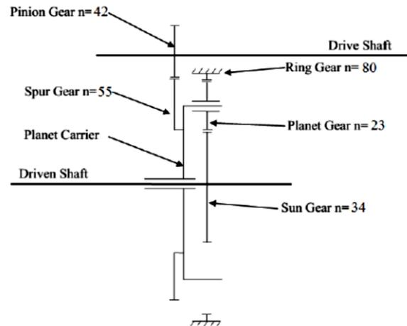
*Figure 2. Test planetary gearbox configuration (Courtesy of UNSW [8])*
