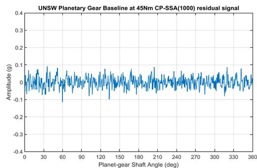
Figure 6. Planet gear residual signal for baseline condition at 45 Nm torque where  $RMS = 0.032(g)$ ,  $Kurt = 2.88$
