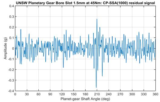
**Figure 11.** Planet gear residual signal for 1.5mm notch at 45Nm torque where  $RMS = 0.0676(g)$ ,  $Kurt = 4.999$
