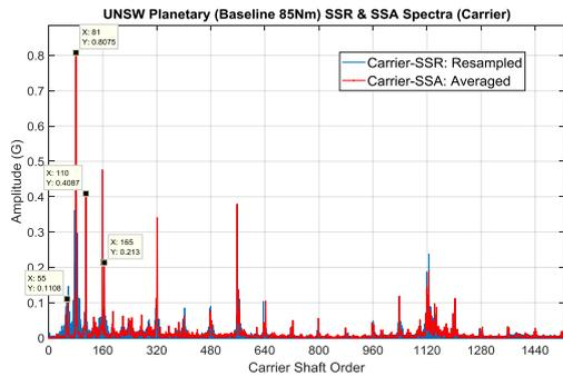
Figure 4. Spectra of the resampled raw vibration signal and carrier-SSA
