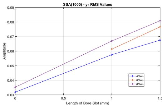
Figure 15. Trending of RMS values of residual signals derived from CP-SSA.
