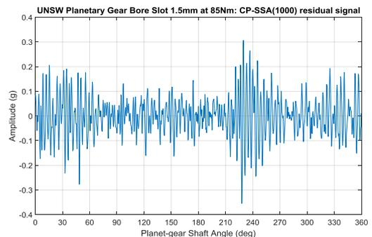
**Figure 13.** Planet gear residual signal for 1.5mm notch at 85Nm torque where  $RMS = 0.0809(g)$ ,  $Kurt = 4.115$
