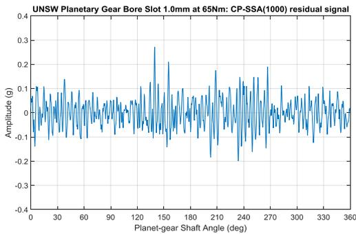
**Figure 9.** Planet gear residual signal for 1.0mm notch at 65Nm torque where  $RMS = 0.0614(g)$ ,  $Kurt = 3.72$
