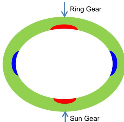
*Figure 23. A diagram showing the opening on tensile stress (red) and the closing on compressive stress (blue) of the bore crack of a planet gear in mesh with the ring and sun gears, respectively.*
