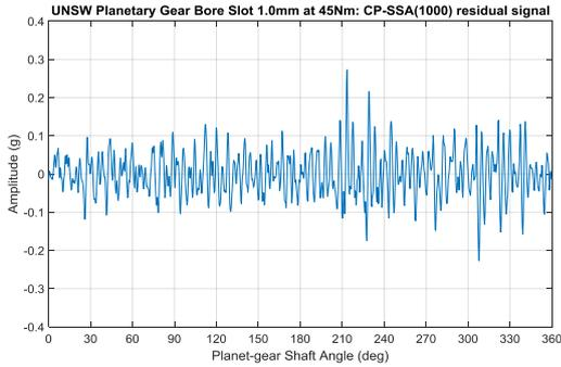
**Figure 8.** Planet gear residual signal for 1.0mm notch at 45Nm torque where  $RMS = 0.0576(g)$ ,  $Kurt = 4.1$
