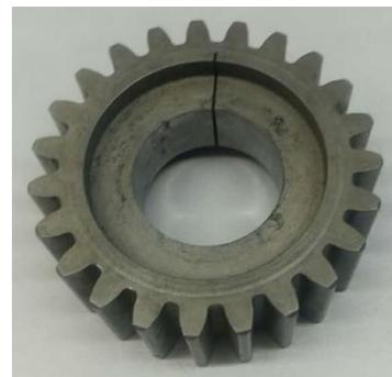
*Figure 3. Test planet gear with an EDM notch (Courtesy of UNSW)*
