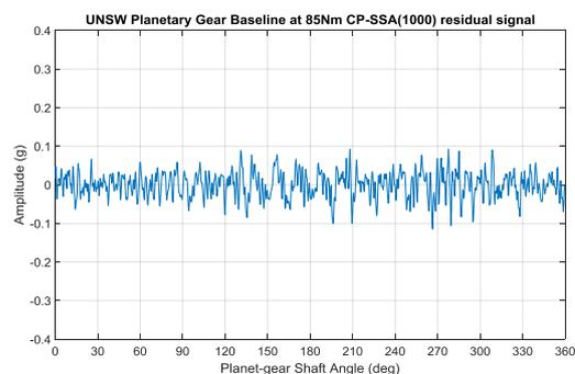
Figure 7. Planet gear residual signal for baseline condition at 85 Nm torque where  $RMS = 0.035(g)$ ,  $Kurt = 3.056$
