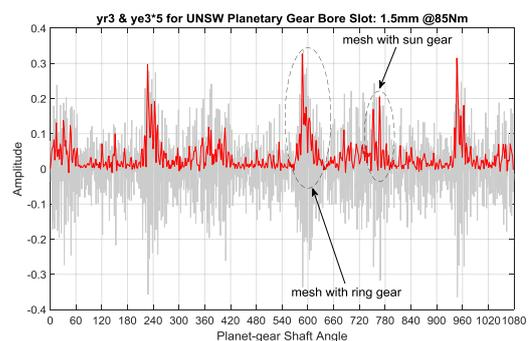
Figure 22. Residual (grey) and scaled envelope (red) signals for 1.5 mm notch at 85 Nm torque
