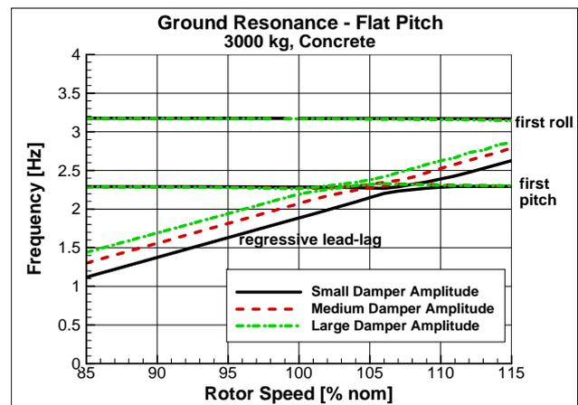
Figure 2: Ground resonance plot: Frequencies
