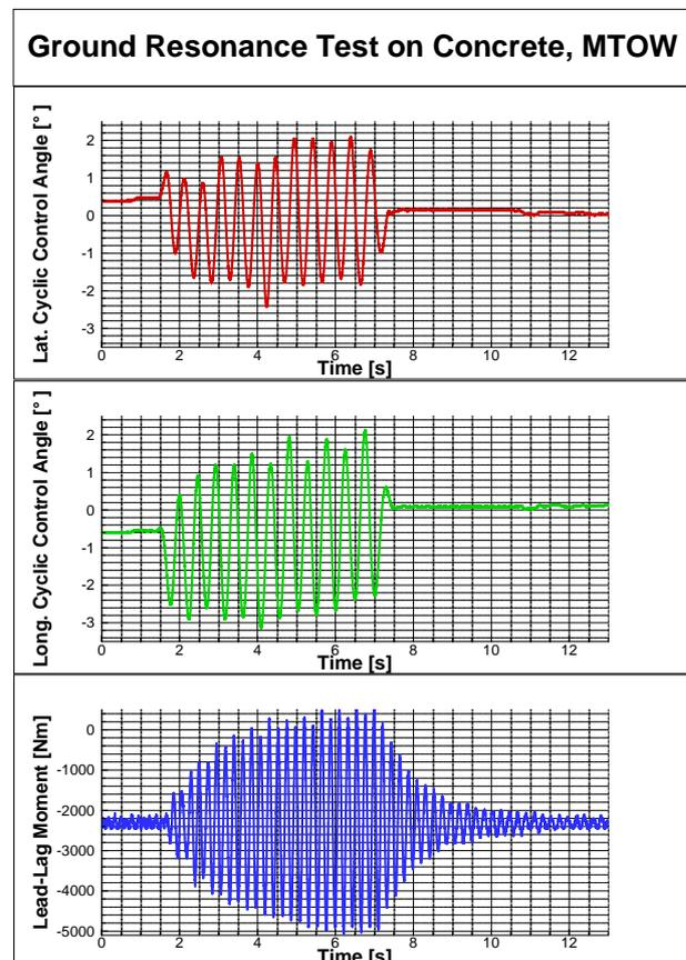
Figure 16: Ground resonance test on concrete
