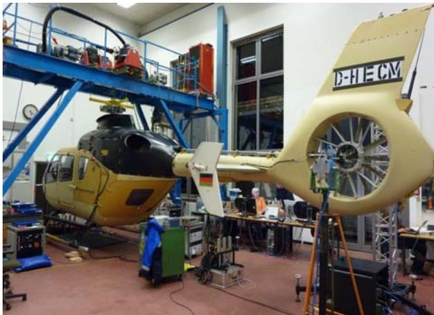
Figure 13: Shake test (© Eurocopter)
