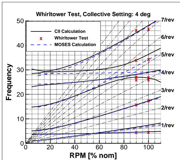
Figure 1: Fan diagram showing calculations and whirtower measurement
