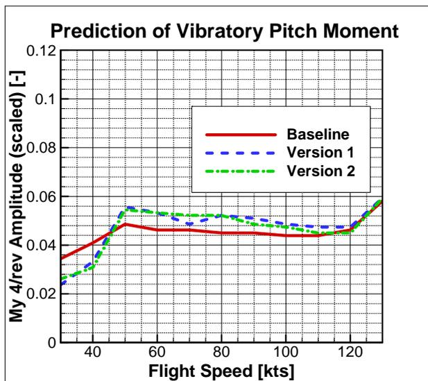
**Figure 4: Vibratory pitch moment (scaled) versus flight speed**
