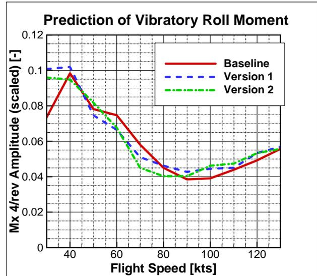
**Figure 5: Vibratory roll moment (scaled) versus flight speed**
