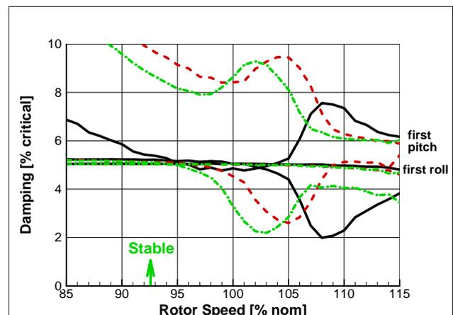
Figure 3: Ground resonance plot: Damping
