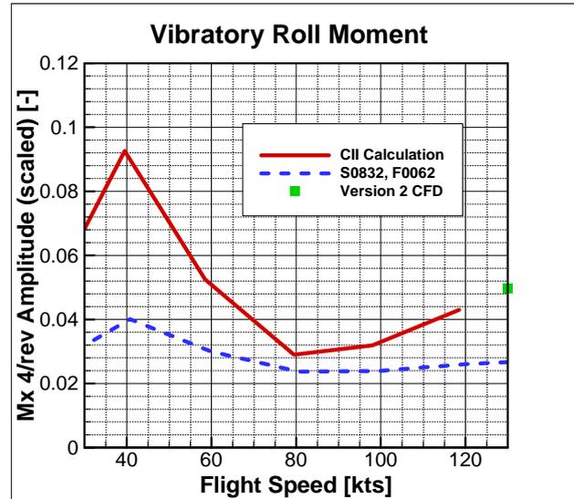
**Figure 8: Vibratory roll moment (scaled) versus flight speed, calculation and measurement**
