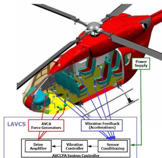
Figure 12: Schematic block diagram of the active vibration control system [5]
