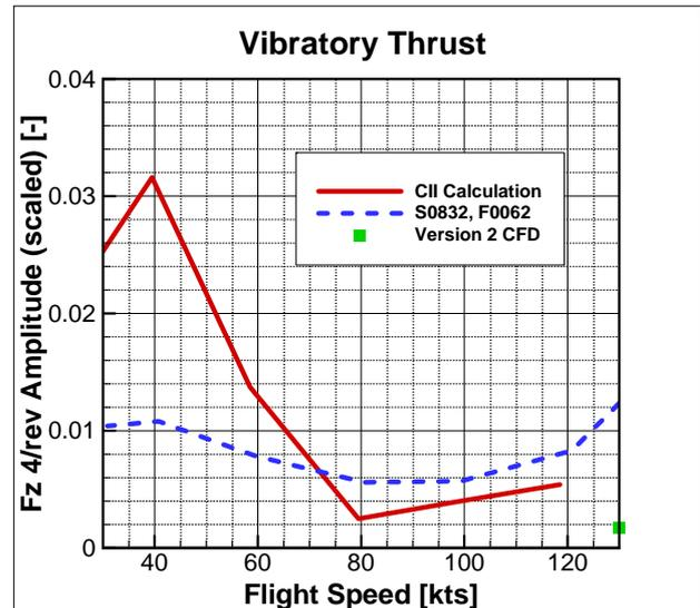
**Figure 9: Vibratory thrust (scaled) versus flight speed, calculation and measurement**
