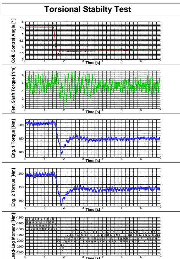
Figure 15: Torsional stability test on ground
