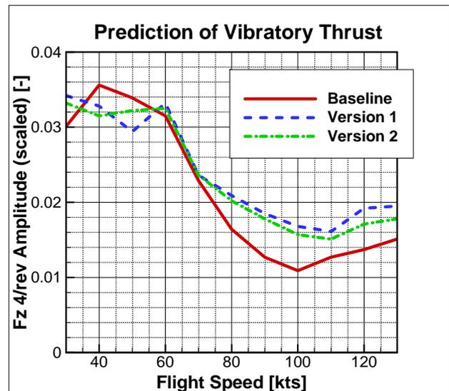
**Figure 6: Vibratory thrust (scaled) versus flight speed**
