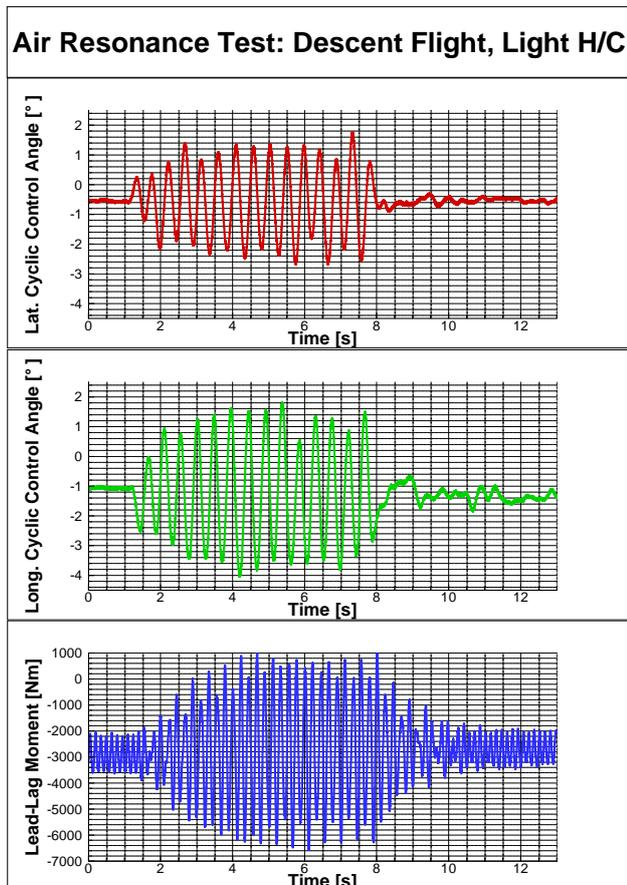
Figure 17: Air resonance test in descent flight condition
