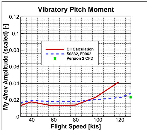
**Figure 7: Vibratory pitch moment (scaled) versus flight speed, calculation and measurement**
