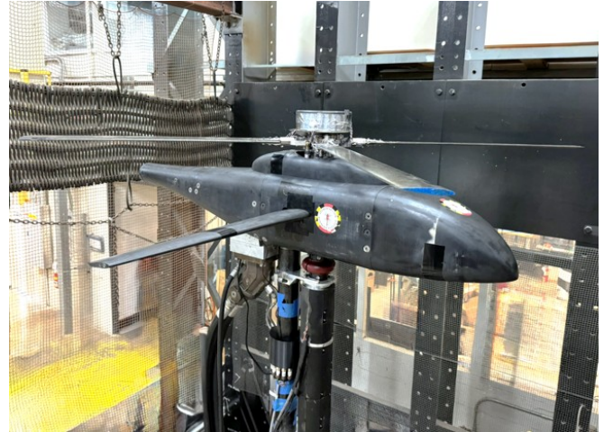
Figure 4. Compound rotor rig with the full wing configuration installed on the UMD hover tower.
