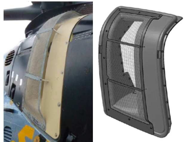
Figure 5: Baseline FOD grid as installed on the H135.
