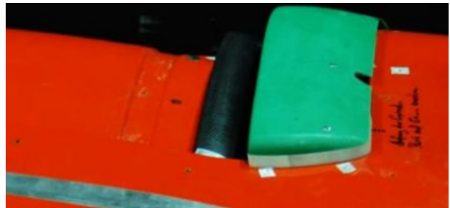
Figure 22: Example of retrofitted add-on on wind tunnel model: high/long rear spoiler with front inlet guide vane, mounted on ramp intake (BSL2-mod) (Ref. 8, fig. 6-b3, page 5).
