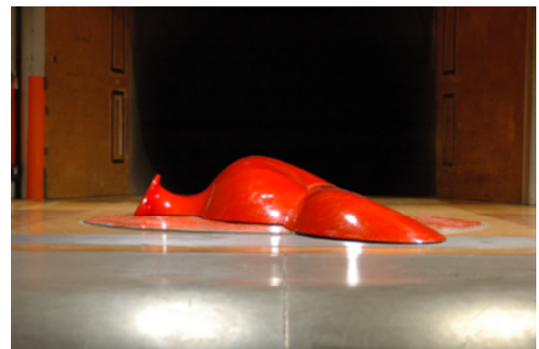
Figure 18: Truncation of the full-scale fuselage (a) (Ref. 8, fig. 2-a, page 3) and fuselage section model in the wind tunnel (b) (Ref. 8, fig. 3-a, page 4).
