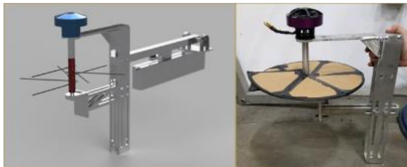
Figure 14: Aerial screw small-scale performance test. Rig design (left) and test setup (right).
