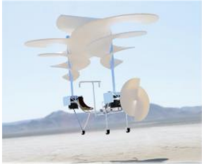
Figure 13 Il Mulinello's lift+cruise aerial screw configuration. Acknowledgements: Thanks to the Georgia Tech Il Mulinello graduate student team: Alex Moushegian (Team Lead), Carlota Bonnet, Alex Markov, and Milad Mozayyani. Team Advisors were: Marilyn Smith and Dimitri Mavris.
