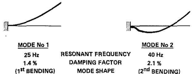
FIG. 1 : NOTION OF VIBRATIONS MODES - CASE OF A CANTILEVERED/FREE BEAM (BENDING)
