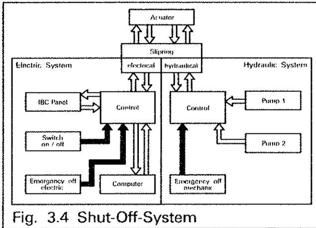
Based on the overall satisfactory results achieved on a test stand, the actuator and the control unit were refined and extended in several stages. Final trials showed a quasi-stationary control operation to be possible with an adequate degree of accuracy, even when the actuator was exposed to high control forces. The final version of the actuator was equipped with an experimental fail-safe-provision which neutralizes the actuator in case of malfunction.
