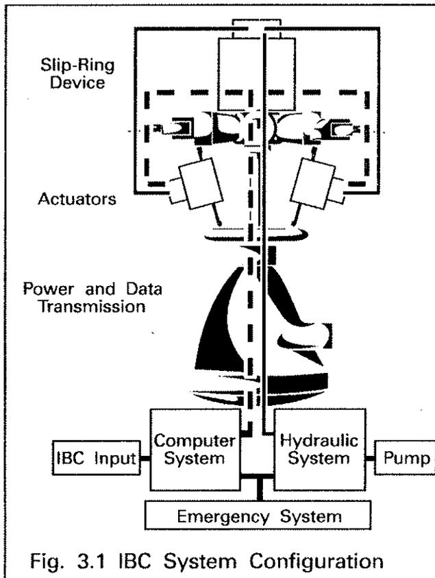
Fig. 3.1 IBC System Configuration
