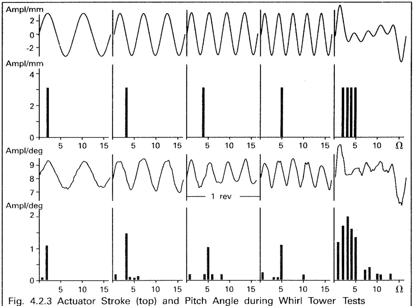
Fig. 4.2.3 Actuator Stroke (top) and Pitch Angle during Whirl Tower Tests
