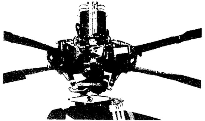
Fig. 4.2.2 Main Rotor with IBC Actuators
