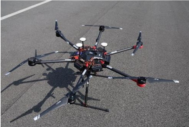
Figure 3: Photo of the DJI Matrice M600 drone with instrumentation
