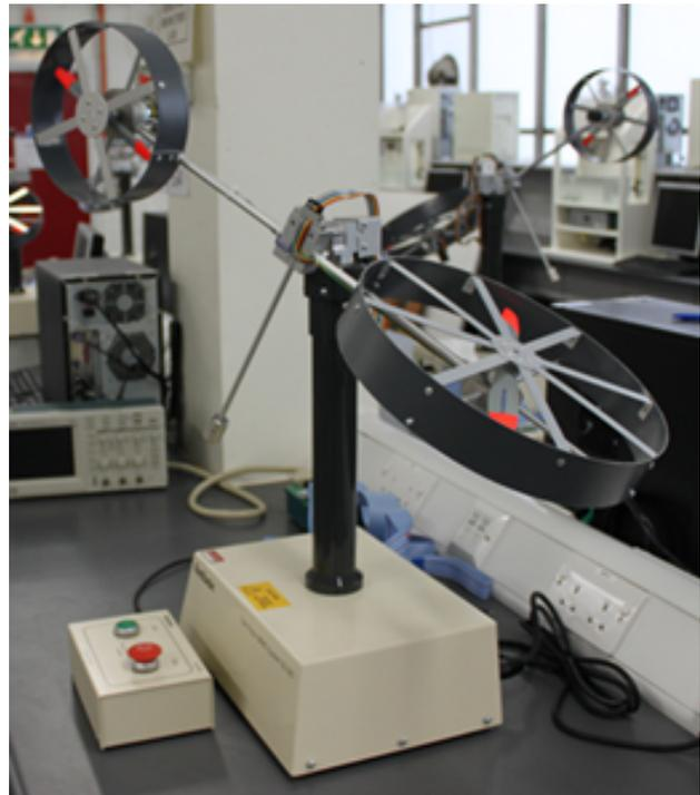
Figure 1: Twin rotor MIMO setup
