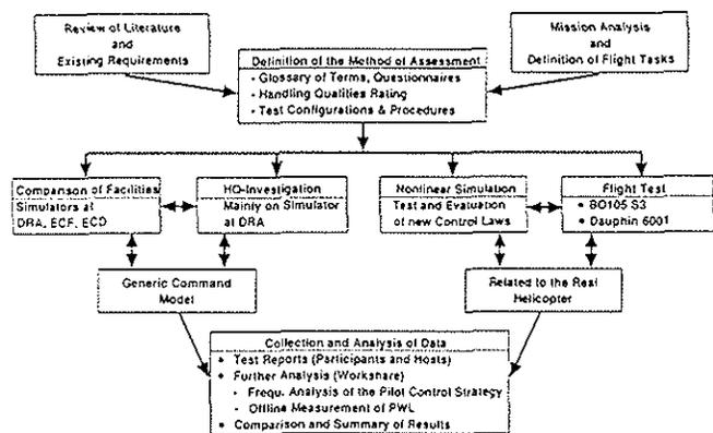
Figure 11: Procedure for the preparation and execution of the trials
