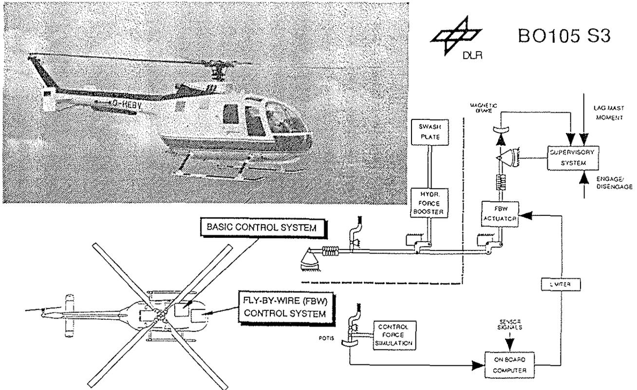
Figure 9: Experimental FBW/L helicopter BO 105 S3
