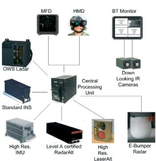
Figure 4: Architecture of the DeViLA concept in phase 3 with an additional OWS ladar sensor used as the basis for synthetic vision display.
