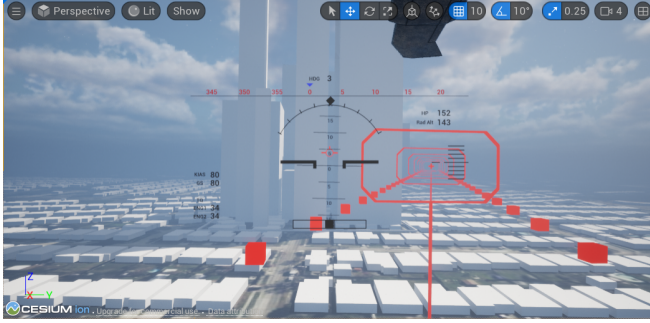
Figure 19. Combination of curved TITS without altitude bar and path marker cubes symbologies, 5 < \tau < 15 .
