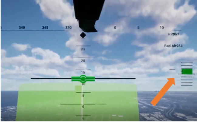
Figure 2. Rate of climb cue shown in a footage of preliminary pilot-in-the-loop testing in the GT high-fidelity, fixed-base rotorcraft flight simulator
