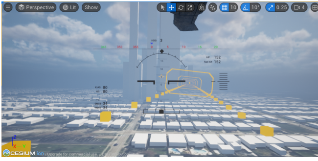
Figure 19. Combination of curved TITS without altitude bar and path marker cubes symbologies, 5 < \tau < 15 .
