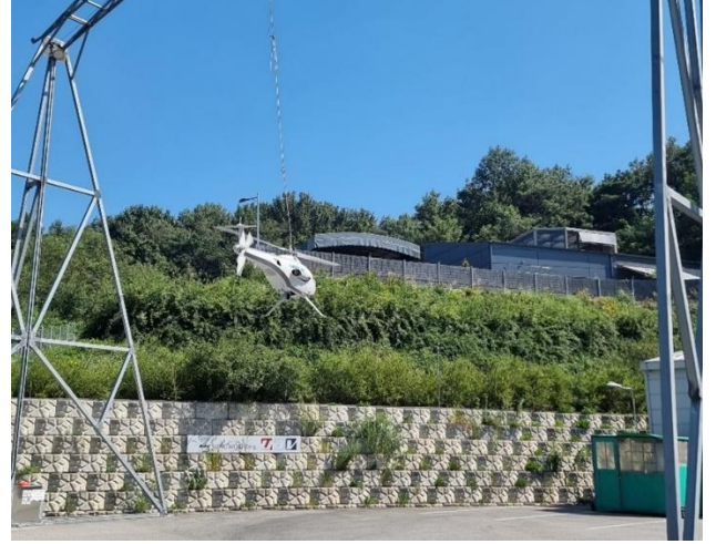
Figure 24: Communication & quasi-flight test of MPUH-C with tethered test setup
