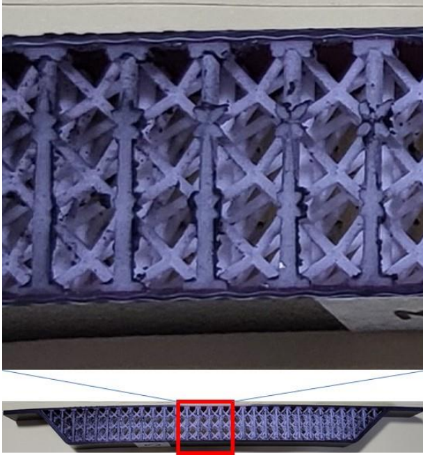
Figure 5: Cutting-section of the CCLAS with 3D printed lattice core
