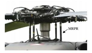
Figure 1. Rotor head of a Black Hawk helicopter.
