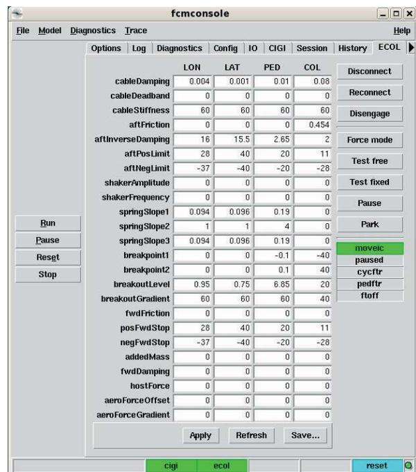
Figure 7 Control Loading Tuning Parameters
