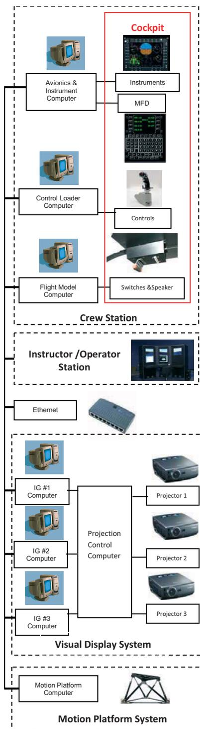
Figure 1: HELIFLIGHT-R Schematic
