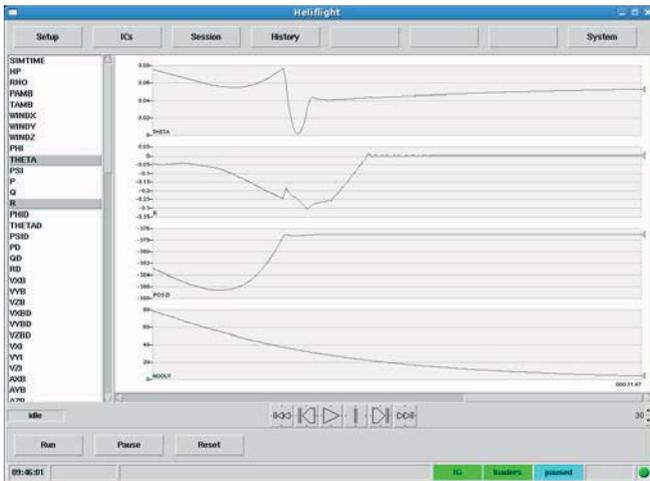
**Figure 5 HELIFLIGHT Run-Time Interface in Data Monitoring Mode**
