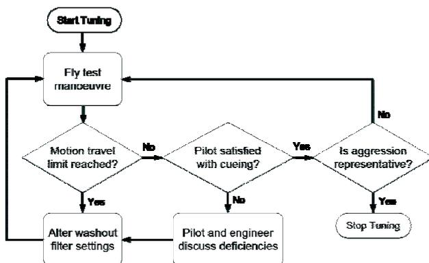
Figure 6 Motion tuning flowchart for one motion axis/manoeuvre
