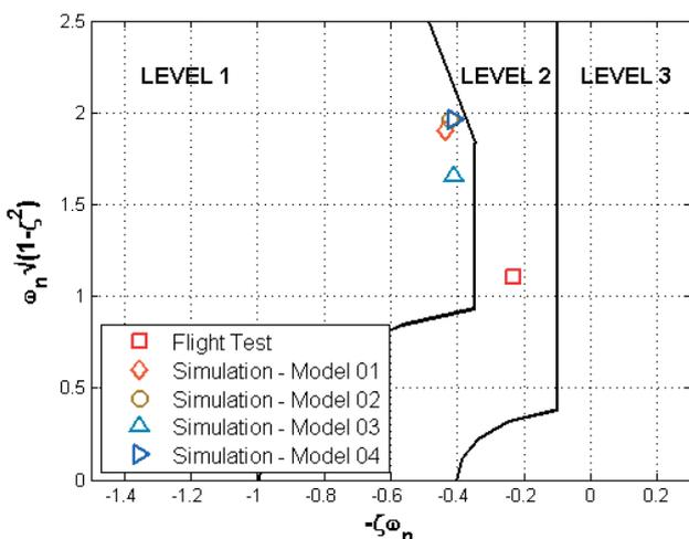
Figure 15: Dutch Roll Stability at 80kts
