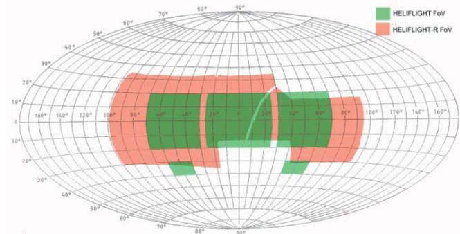
**Figure 4: Comparison of Outside World Field of View Between HELIFLIGHT-R (Left hand Seat) and HELIFLIGHT simulators.**
