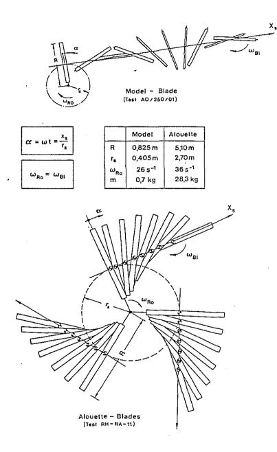
Figure 2. Rotor Blade Removal from Tethered Helicopter (Comparison Model Helicopter-Alouette Helicopter)
