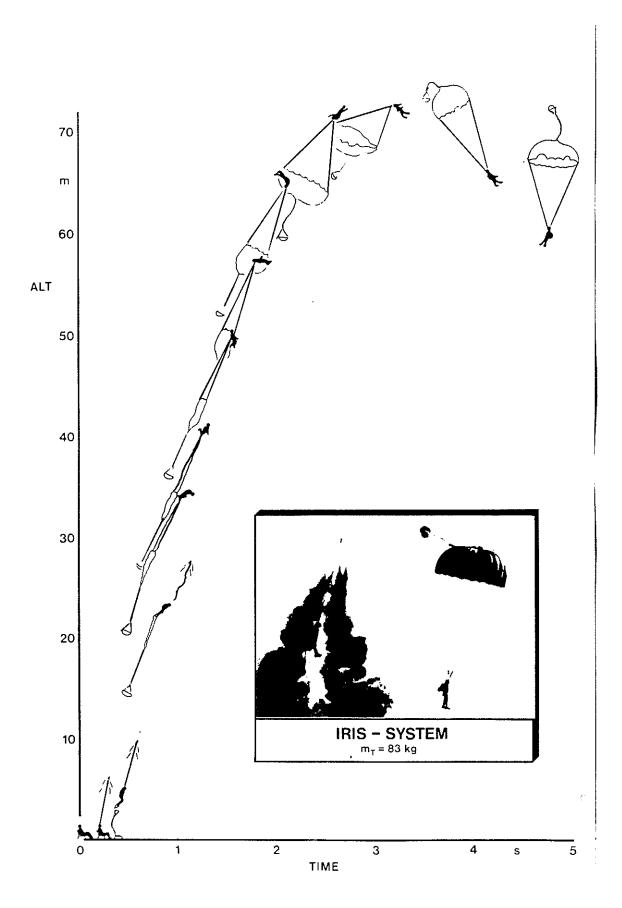
Figure 4. IRIS: Altitude vs. Time during o/o-Test
