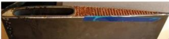
Figure 2: Cross section of UH-60A rotor blade[12]
