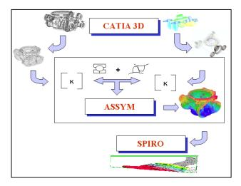
Thanks to the advances integrated in ASSYM and in design software, such as CATIA®, it is now possible in this new step to design and model all the parts in 3 dimensions, regardless of their complexity.
