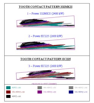
Once determined, these parameters will accurately produce the simulated tooth surface. <u>Tooth contact pattern under load</u>
