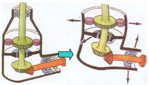
The casing deformations can reach several millimeters. They interfere with the functioning of the mechanical contacts, which in service immediately leads to flaking and scratching on the teeth.
