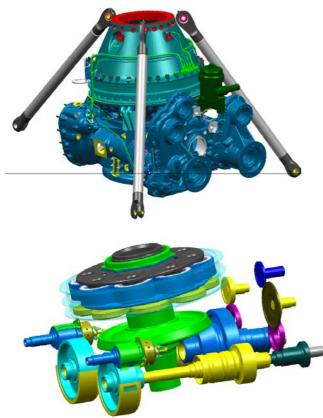
One of the main differences between the 332 MKII and the EC225/725 MGBs is the bevel gear drive.
