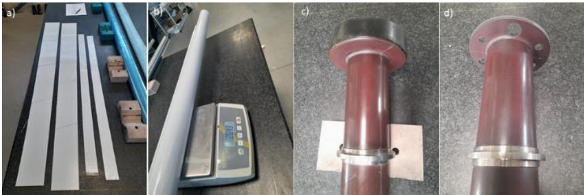
Figure 11: Four steps of material evolution from a ply to a final composite shaft
