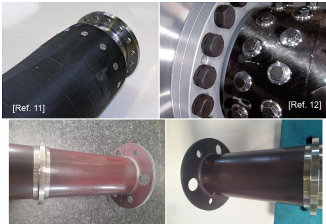
Figure 1: Comparison of an integrated metallic flange (top two images) and a fully composite flange (bottom two images)
