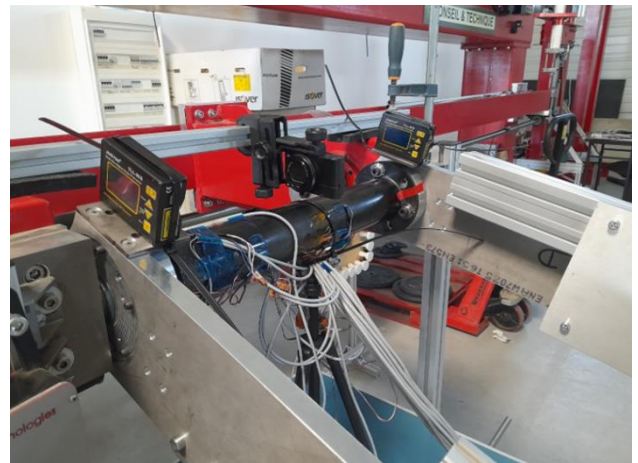
Figure 9: Torsional bench setup with shaft S5
