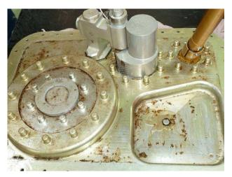
Figure 8 Damage of a fuel equipment plate due to Bio-contamination
