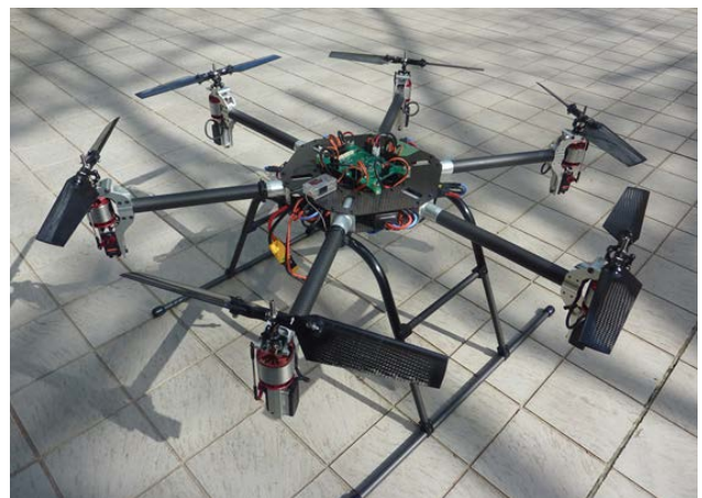
Figure 1: A variable pitch control hexa-copter
