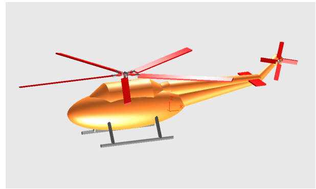
Figure 1: The five-bladed dynamic helicopter demonstrator H9 with articulated rotor — side view
