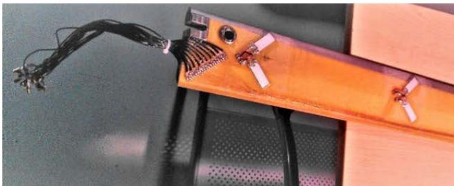
Fig.3. Allocation of vibration deformation sensors on low pressure (a) and high pressure (b) surfaces of the blade.
