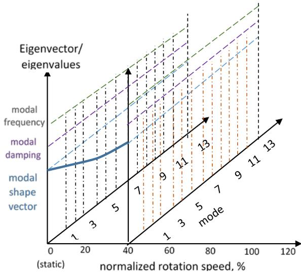
Figure 1. Graphic illustration of typical modal passport structure
