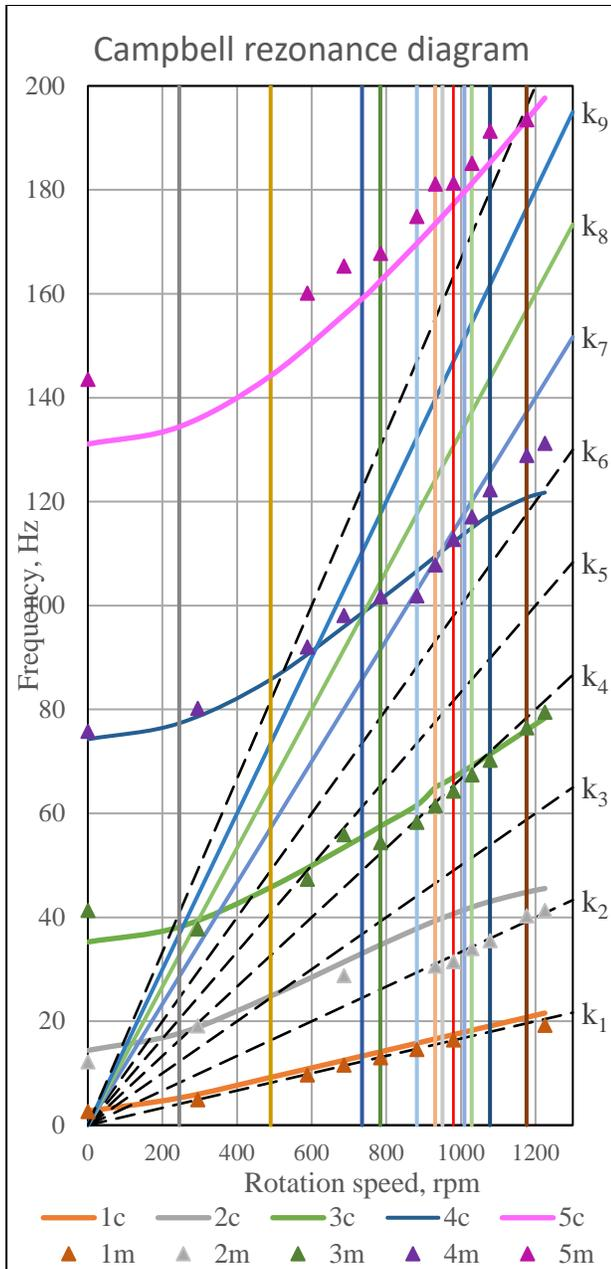
Figure 11. FEM computed and experimentally measured modal frequency dependence on normalized rotation speed.
