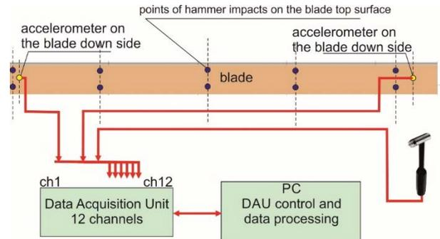
Figure 7. Measurement setup of blade testing by roving hammer technique.
