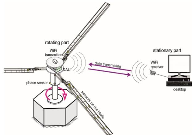
Figure.2. Setup of rotating blades measurement system
