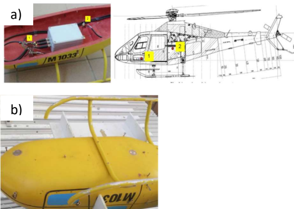
Figure 7: Sensor location a) accelerometers b) pressure. Credits: CTO/ PZL-Świdnik
