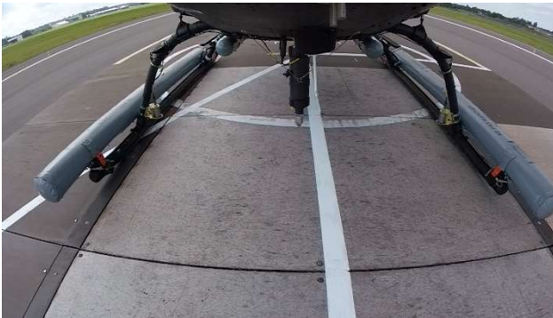
Figure 43: SW-4 SOLO landing approach on the moving platform with anchor mock-up device. Credits: PZL-Świdnik
