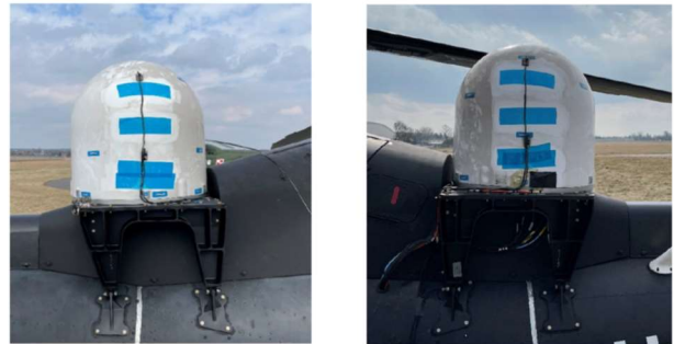
Figure 14: Antenna installation – right and left side view. Credits: PZL-Świdnik
