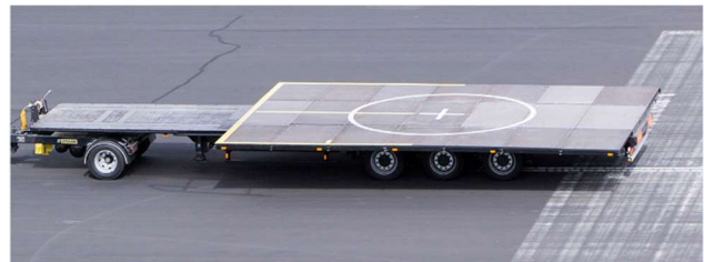
Figure 42: Moving platform to simulate SW-4 SOLO landing scenarios on vessel. Credits: PZL-Świdnik
