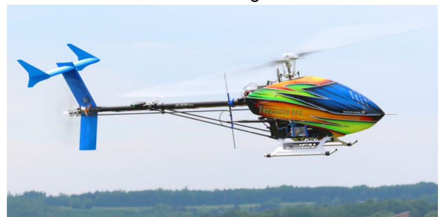
Figure 3: UAV testbed with modified tail section. Due to the phase shift of the rotor, a side mounted wing does not lead to the desired unloading of the retreating blade.
