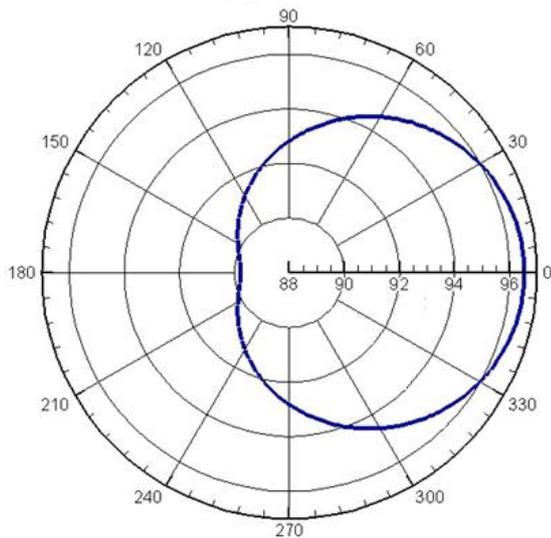
Figure 12 – Diagram of sound emission directivity in horizontal plane, SPL (dB)
