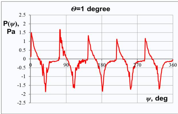
Figure 5 – Sound pressure oscillation,  $\theta=1^\circ$
