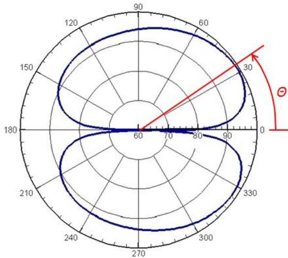
Figure 11 – Diagram of sound emission directivity in vertical plane, SPL (dB)
