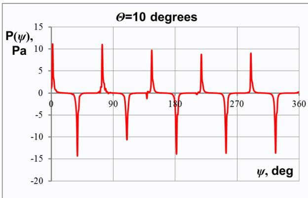
Figure 6 – Sound pressure oscillation,  $\theta=10^\circ$
