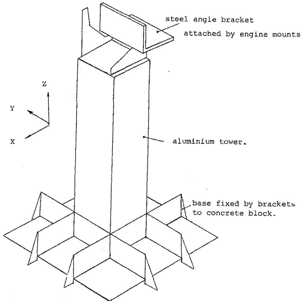
Diagram of TOWER STRUCTURE with steel angle bracket.
