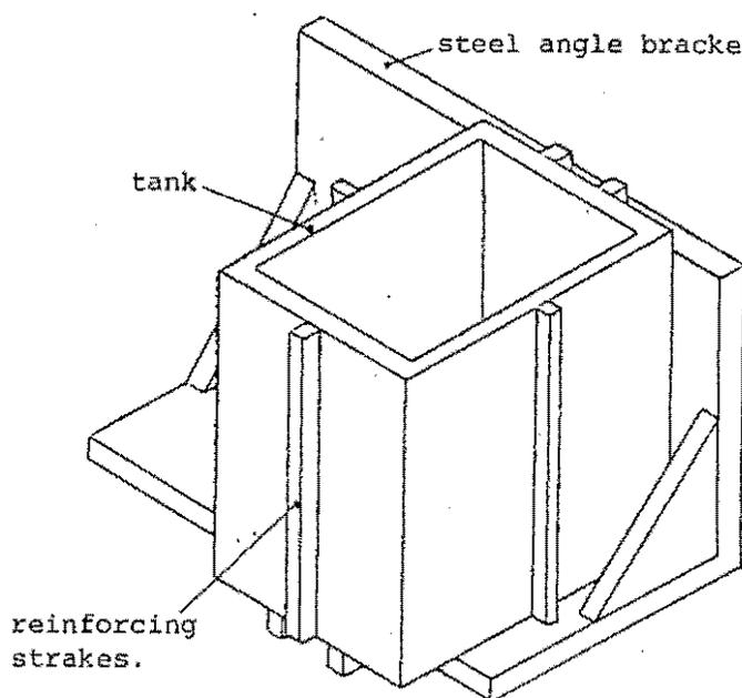
Diagram of steel tank bonded to steel angle bracket.
