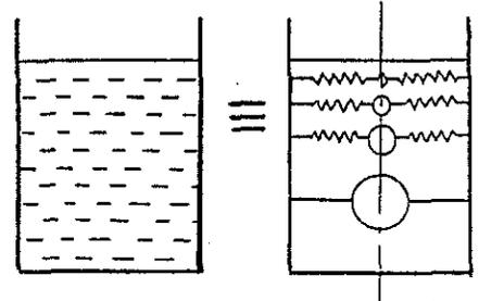
Equivalent spring and mass model of fluid for sway motion.
