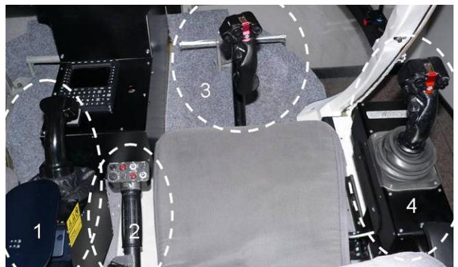
Figure 3: Assembly of left hand (1) and right hand sidestick (4) and conventional inceptors (collective (2), centrestick and pedals (3)) in the helicopter simulator
