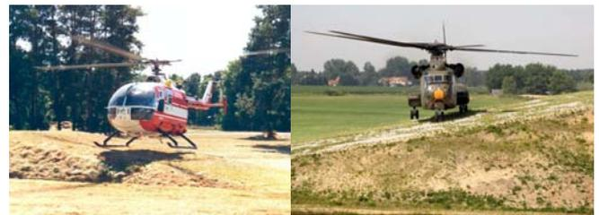
**Figure 13: The Bo-105 S3 and a CH53 demonstrating slope landings**
