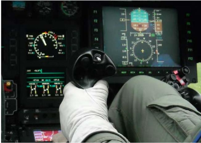
**Figure 11: Cockpit with PFD (right), limit indicator display (left) and collective sidestick (front)**
