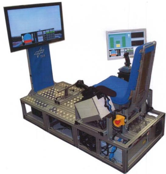
**Figure 20: Technology demonstrator for rapid prototyping of tactile pilot assistance**
