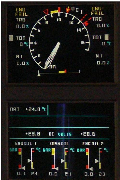
**Figure 12: VEMD (Vehicle and Engine Monitoring Display)**
