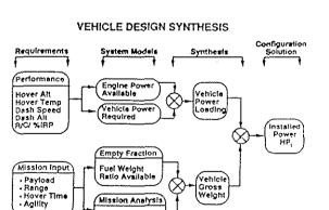
Fig. 1 Vehicle Design Synthesis
