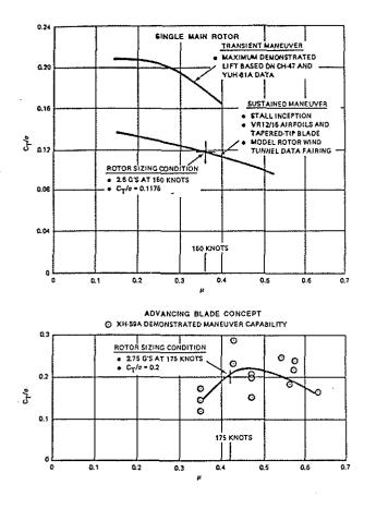
Fig. 9 Maneuver Rotor Lift Boundaries
