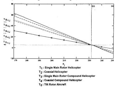
Fig. 6 Hovering Time vs. Range (4000 ft/90 deg.)
