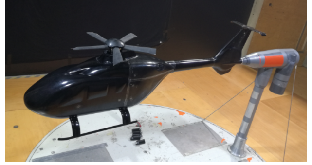
Figure 1. Helicopter model with rotor head variant R1 in the wind tunnel test section.
