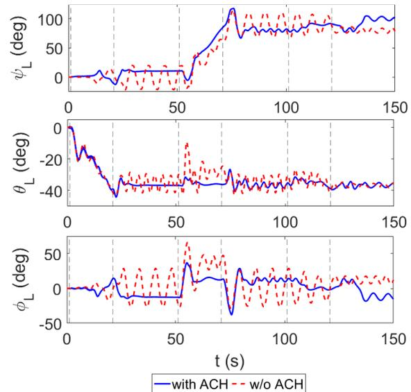
Fig. 20. Load attitude angle during a complex maneuver
