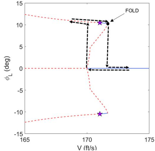
Fig. 14. Controlled system instability near fold, 101 kt (170.5 ft/s)
