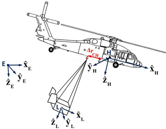
Fig. 3. Coupled helicopter-external load system
