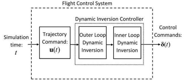
Fig. 2. Helicopter flight control system model
