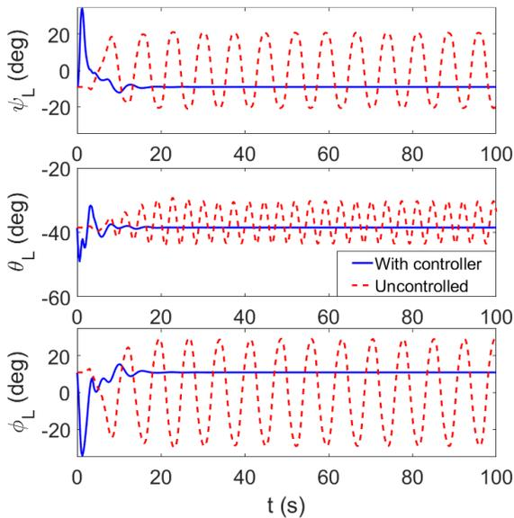
Fig. 8. Solution trajectories of the controlled and uncontrolled systems, 100 kt (168.8 ft/s)
