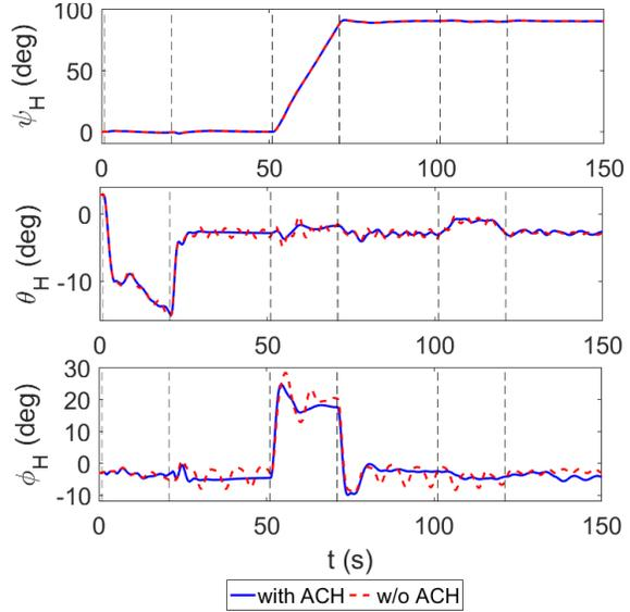
Fig. 19. Helicopter attitude angle during a complex maneuver
