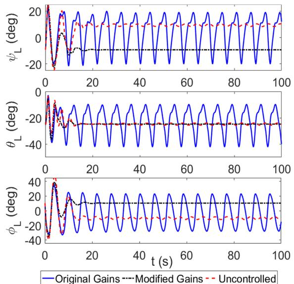
Fig. 12. Effect of gain modification, 75 kt (126.6 ft/s)
