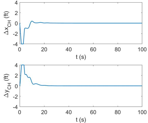
Fig. 9. Cargo hook displacement following load excitation, 100 kt (168.8 ft/s)
