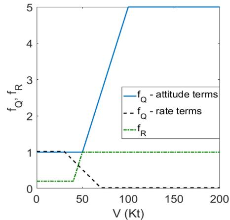
Fig. 11. Airspeed scaling of weight matrices
