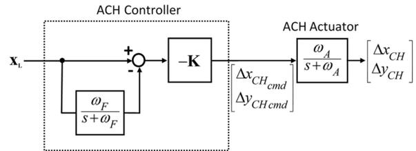
Fig. 7. Active cargo hook LQR controller and actuator models
