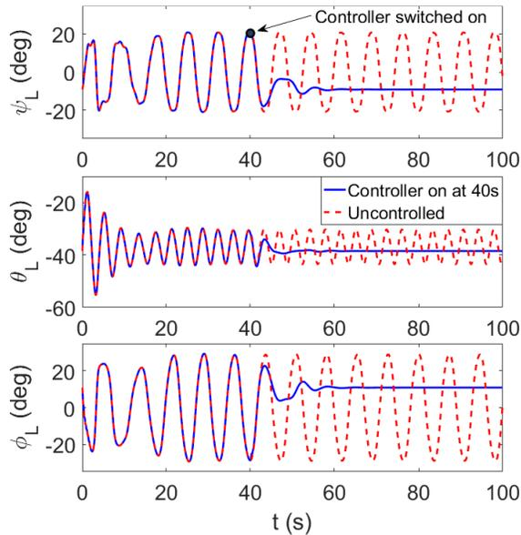
Fig. 10. Solution trajectories following controller switch on at 40 s, 100 kt (168.8 ft/s)
