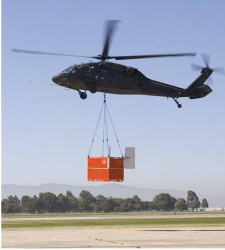
Fig. 1. Test helicopter carrying the fins-stabilized CONEX cargo container [15]
