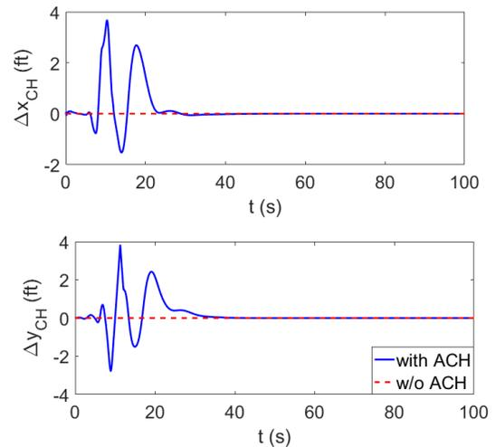
Fig. 18. Cargo hook stroke, 97 kt (163.8 ft/s)
