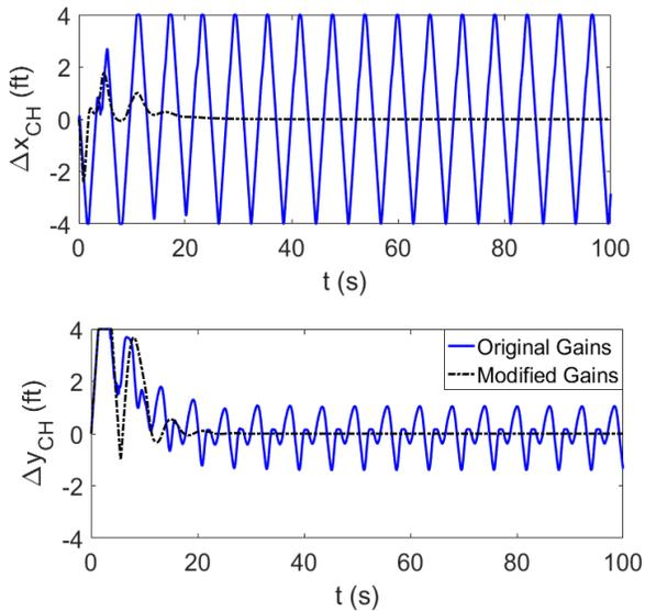
Fig. 13. Cargo hook stroke, 75 kt (126.6 ft/s)
