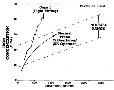
Fig. 2 Main Rotor Gearbox — Case History 1 (Light Pitting)
