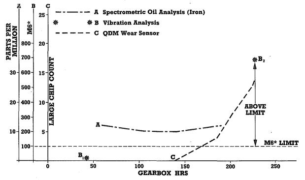
Fig. 3 Main Rotor Gearbox — Case History 3 (Tooth Fracture)
