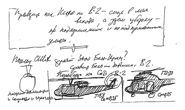
Fig. 2. Comparison of the V-2 and Bell Iroquois in terms of aerodynamic drag, 1964.
