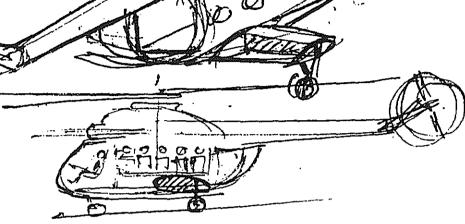
Fig. 3. Possible fuselage changes in case more powerful engine are installed, 1965.
