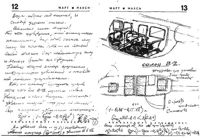
Fig. 1. The derivation of the relationship between weight efficiency and engine power and main rotor diameter (on the right) and the V-2 passenger cabin layout (on the left), 1964.
